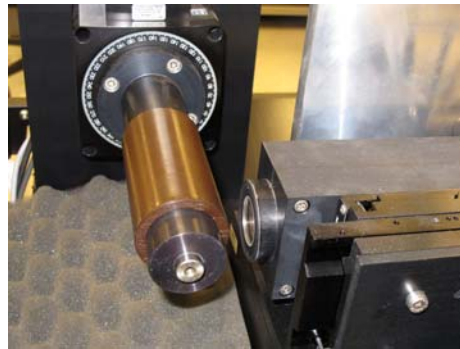
Figure 3: Overall view of the present full scale 3D cylinder scanner. Cylinder, in foreground, is held on mandrel and rotated by stage (marked with circular scale). Probe enters from right and is held on linear translation stage (lower right). Laser displacement sensor scans cylinder from above (marked with yellow safety tag).
