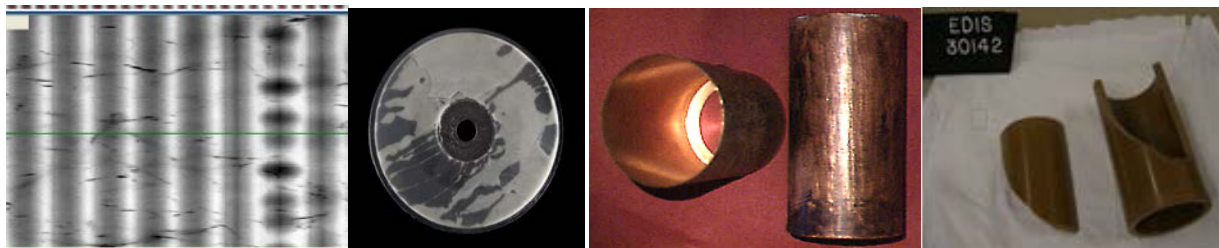
From the left (a) Depth image from wax cylinder showing damage from fibers on the surface (~1910). (b) Experimental recording, wax on paper, Smithsonian (A.G. Bell, early 1880's) (c) Copper cylinder “galvano” mold (early 20th century). (d) The Dickson Cylinder from Edison National Historic Site (1893).
