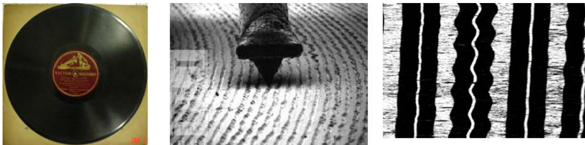
Figure 2: Historical disc records, composed of shellac, wax, plastic, lacquer, or metal carry sound in a spiral groove which undulates laterally in the surface plane. Typical groove width is 150 microns
