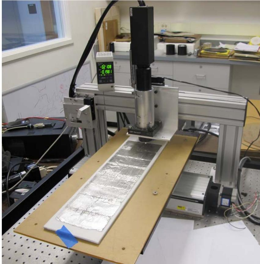
Figure 2: The Berkeley Lab optical scanner holding the 1878 St. Louis tinfoil. The foil is mounted on the flat bed of a computer controlled, two axis movement. One of the scanning stages can be seen protruding from under the bed at right. The optical probe used is the vertically mounted black and metallic object at the center. A light spot can be seen just at the top of the foil.
