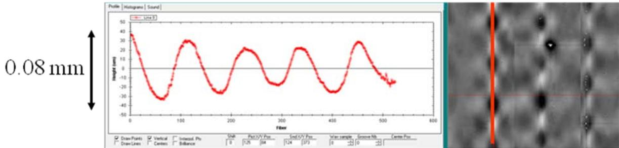
Figure 4: A different view of the foil surface. Here the red line runs in the direction of the audio track. The recording and playback stylus would move from top to bottom in this image. The reconstructed stylus motion is shown at left.
