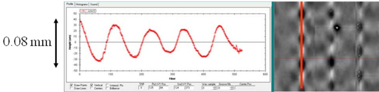
Figure 4: A different view of the foil surface. Here the red line runs in the direction of the audio track. The recording and playback stylus would move from top to bottom in this image. The reconstructed stylus motion is shown at left.
