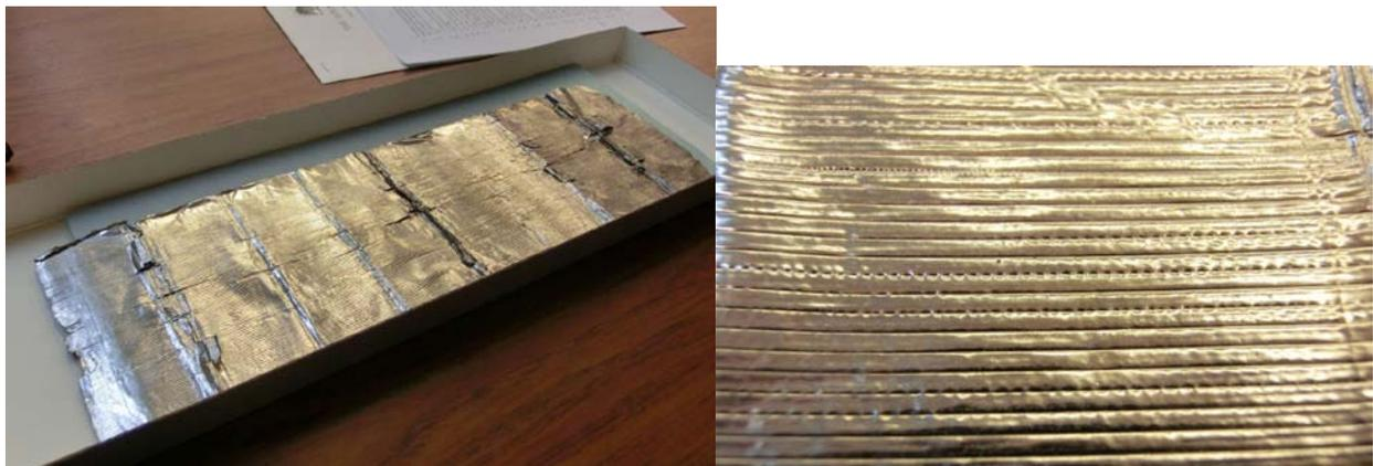
Figure 1: Top left is a sketch from Edison's patent application for the Phonograph. A reconstruction of the original device is at upper right. The 1878 St. Louis tinfoil is at lower left with a detail shown at lower right. The multiple fold marks are visible as well as the detailed groove structure carrying the embossed audio pattern.
